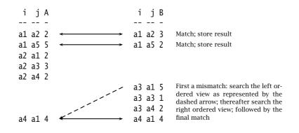
Figure 12.2: Sparse execution of the \* operator
