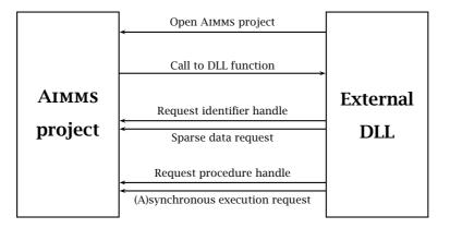
Figure 34.1: Interaction between AIMMS and an external DLL
