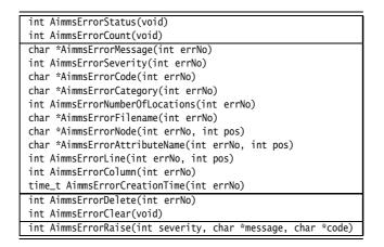
Table 34.7: AIMMS Raising and handling errors in the AIMMS API
